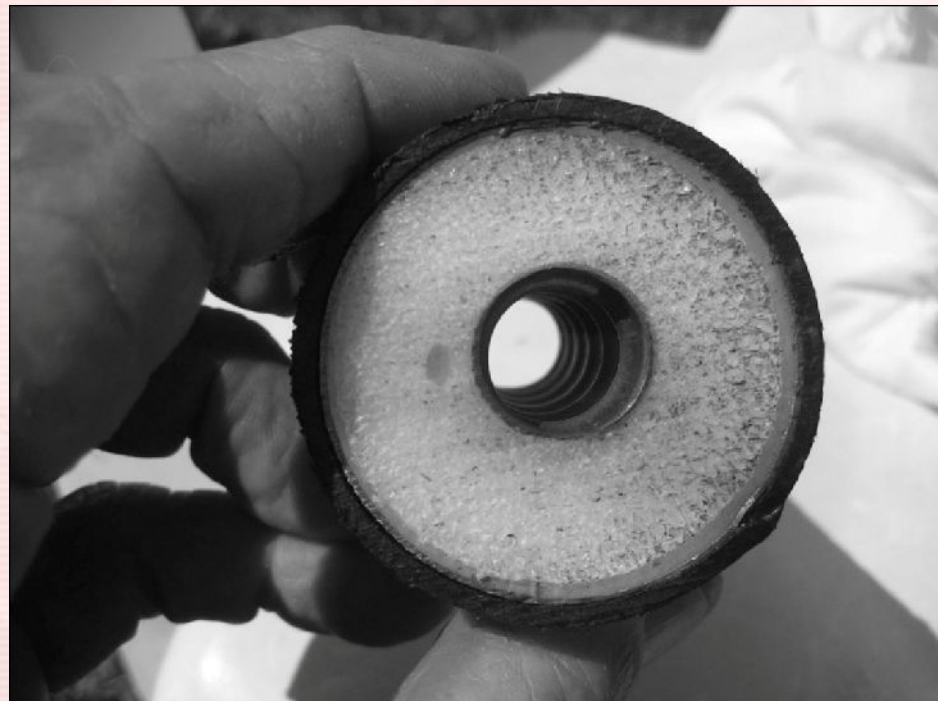
Large coax, with hollow center conductor, low loss
